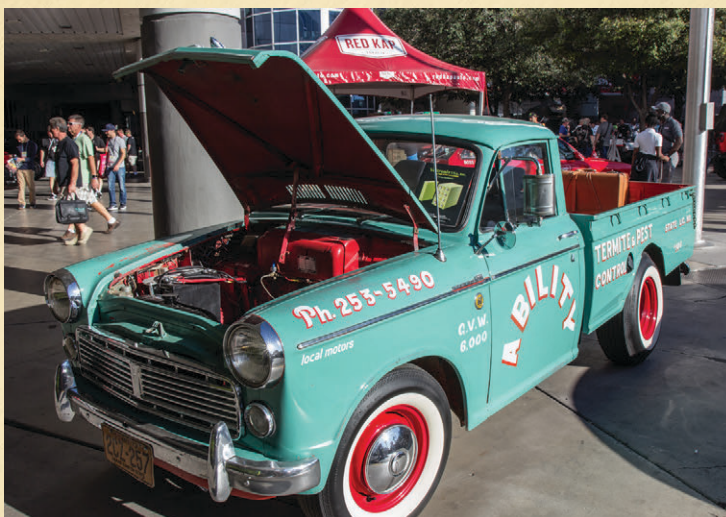
A truck deserving a double take was this Datsun 1200 that showed off the empty engine bay which got you scratching your head. In the bed revealed the electric power plant powering this classic pickup.
