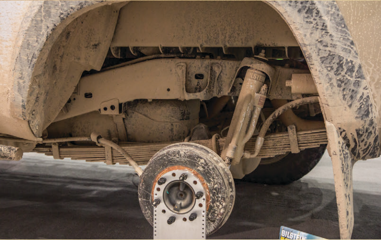
Bilstein had some tricks up their sleeves, well behind their wheels, on their Tacoma build this year. New bypass rear suspension accompanied new coilovers featuring ZoneControl dampening.
