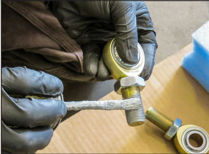
We coat the rod ends with silver anti-seize.
