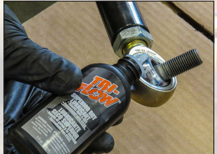
Before you install the rod end boots, make sure to put some Tri-Flow on the joints. You can use the UCA bolt to move the ball from side to side and work the Tri-Flow into the joint.
