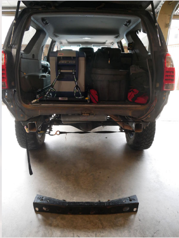
Crossmember removed and three inches cut off of the rear frame.
