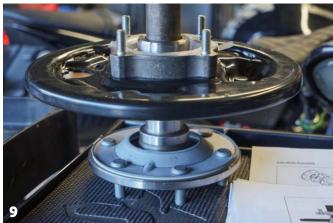
On to the home stretch! Using a couple press tools and a press, press the retaining ring and bearing assembly onto the shaft. When pressing on the unit bearing, take note of the black ring. This is the ABS tone ring and can easily become damaged. If you have a pressure gauge on your press, the gauge will begin to spike when fully compressed. If no gauge, you'll have to use best judgement to determine when the assembly is fully pressed in. **[10]**
