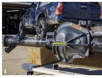
.313" wall DOM tubing, stock width, leaf spring perches and factory location shock mounts. Dynatrac includes their beefy 35-spline 1.5" diameter, semi-float, USA-grade 1541H alloy axle shafts with a 6 on 5.5" bolt pattern. The ProRock 60 is setup to house a massive 9.75" ring gear and contains their Dual Sump High Volume lubrication system for optimal oiling. The housing and shaft kit will set you back \$3,999 plus taxes and shipping. **[2, 3]**
