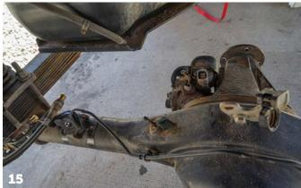
are draining out. At this time, you can swap in a new gasket or apply new gasket maker. I have been using a Lube Locker gasket, so I do not have to mess with gasket maker anymore. **[21]**
