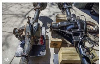
hole that will need some attention as well. Once the rear hole has stopped flowing out, you'll need to add some additional oil in the forward fill hole. You will add oil until it begins to flow out the main fill hole again. Give it a few minutes to finish leveling itself out inside and plug the fill holes back up... **[24]**
