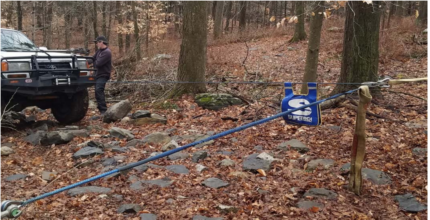
Figure 8: Synthetic winch rope with a roller fairlead.
