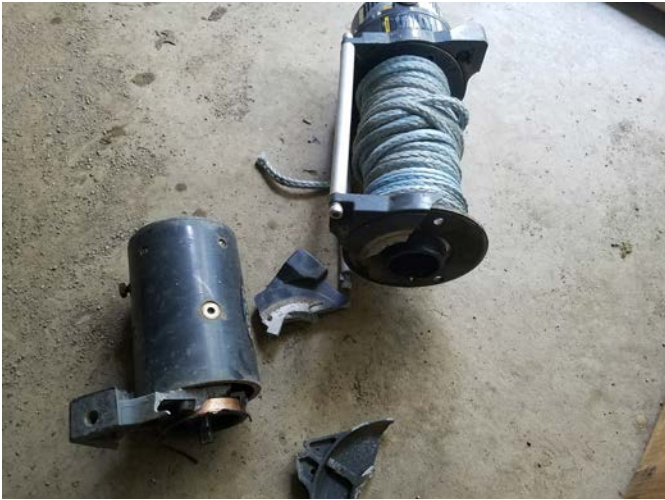
Figure 4: Cast housing failures are rare, but in extreme duty circumstances, can happen.
