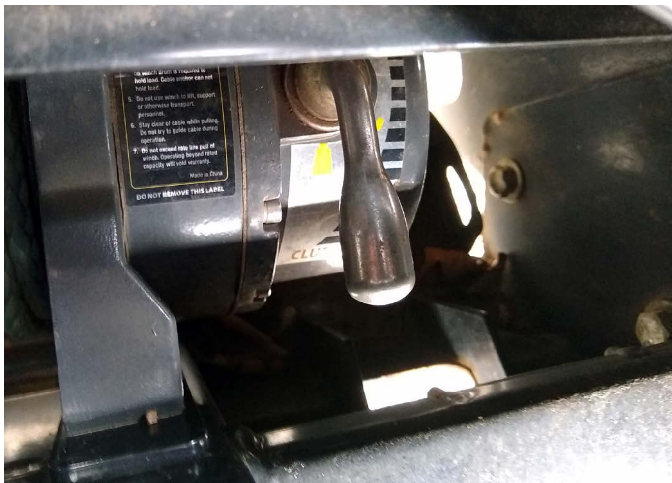
Figure 9: This installation of a winch into a bumper was foot forward, therefore the winch had to be clocked to line the clutch lever up with the small access hole – and it’s still not easy to get to!
