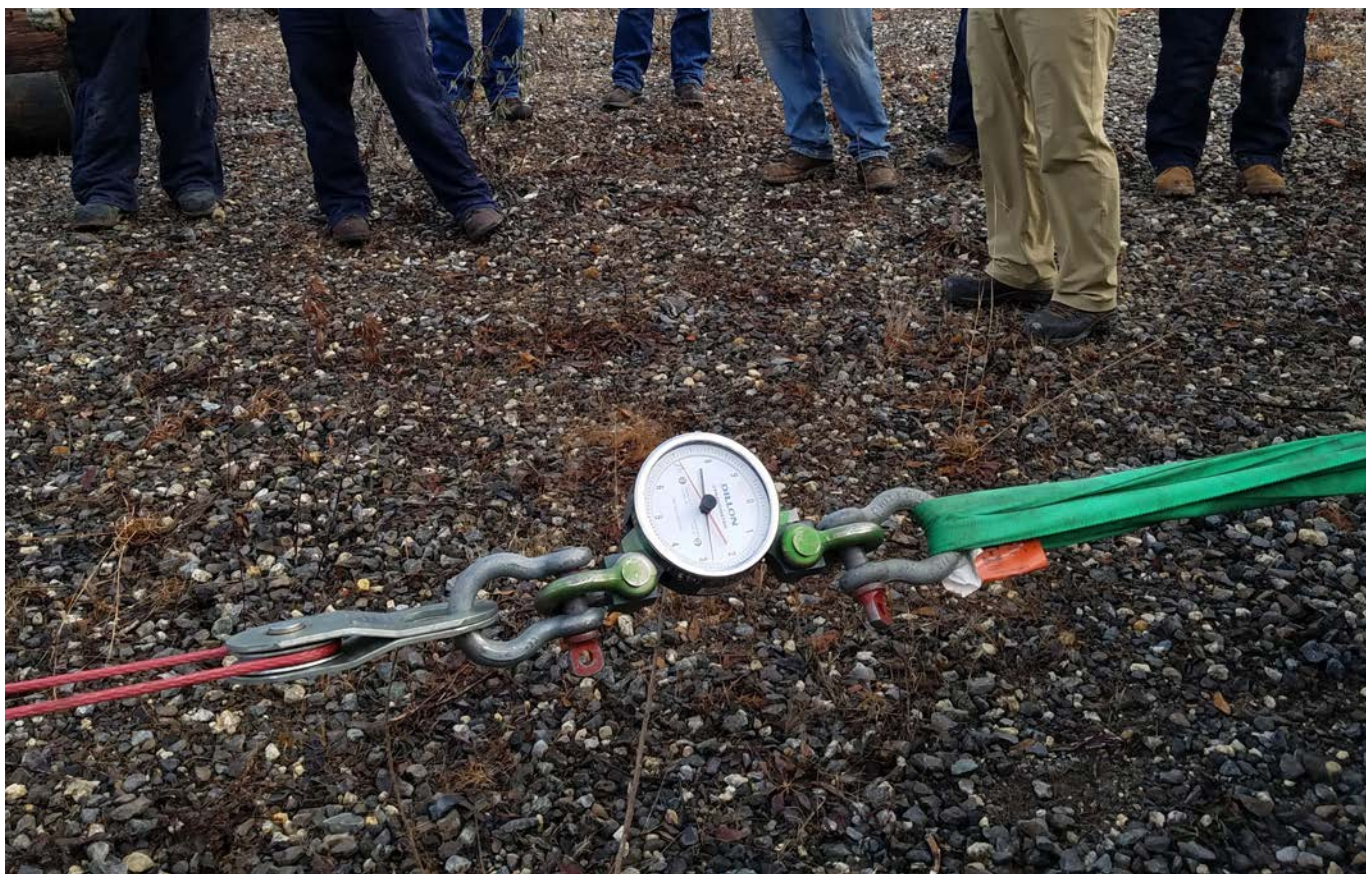
Figure 2: Measuring winch pulling power using a dynamometer
